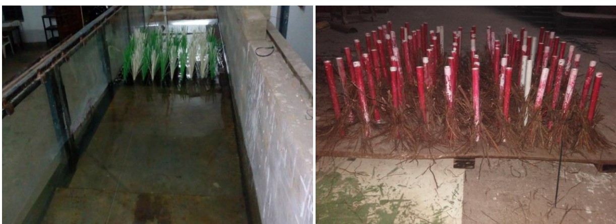
Figure.3. Flexible and rigid vegetation with roots model fixed in a 2-D wave flume
