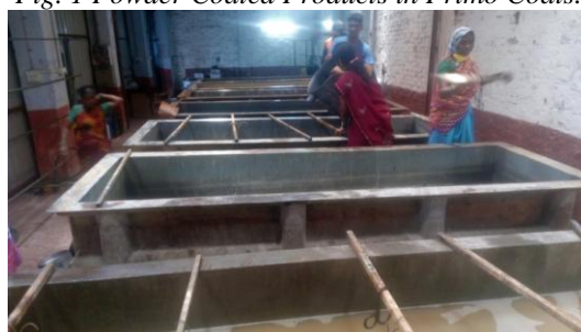
Fig.2 Manual Pre-Treatment process at Primo Coats.
