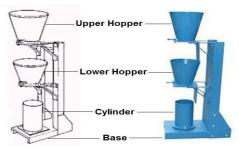
**Compaction Factor Test on Concrete**
