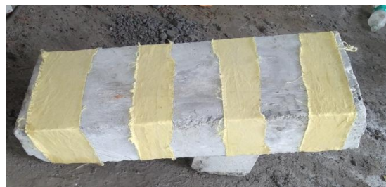
figure 4 80mm strip wrapping of aramid fiber
