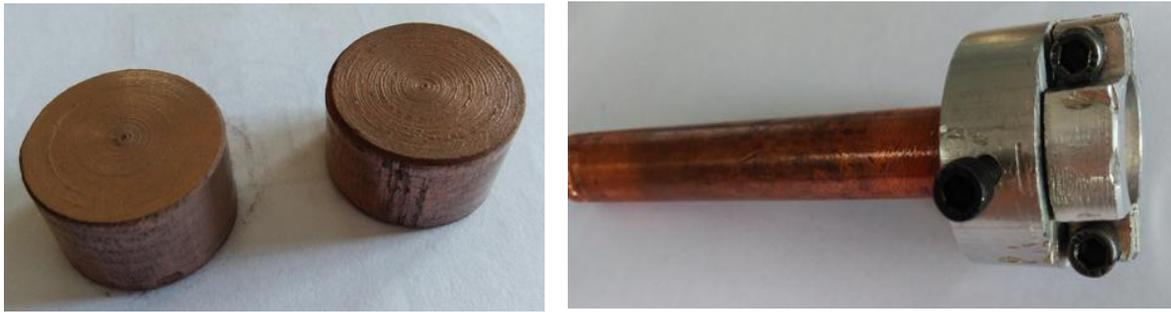
*Fig. 1 P/M Tool electrode and Tool clamping extension*
