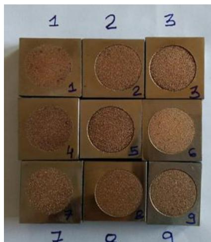
*Fig. 2 EDMed workpiece of P20+Ni using P/M electrode*
