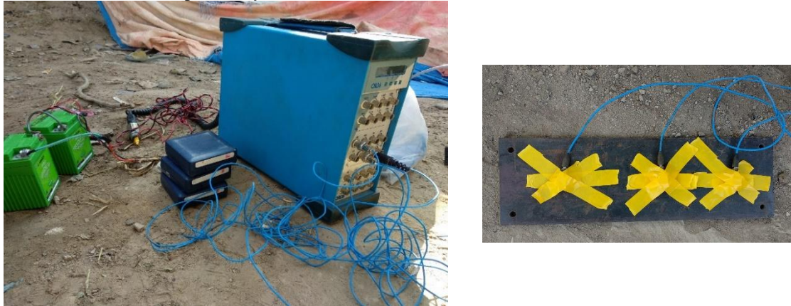
Figure 4 Instrument setup: OROS OR36 Analyzer
