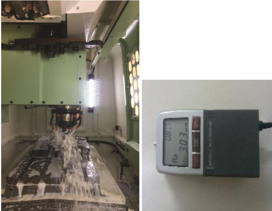
Figure 2: Detailed view of end –mill and work piece setup Figure 3: Mitutoyo Surf test SJ-201P
