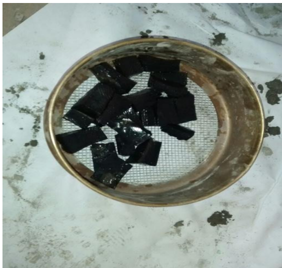
Figure 1: NaOH treated rubber. Figure 2: Cement paste treatment given to rubber.
