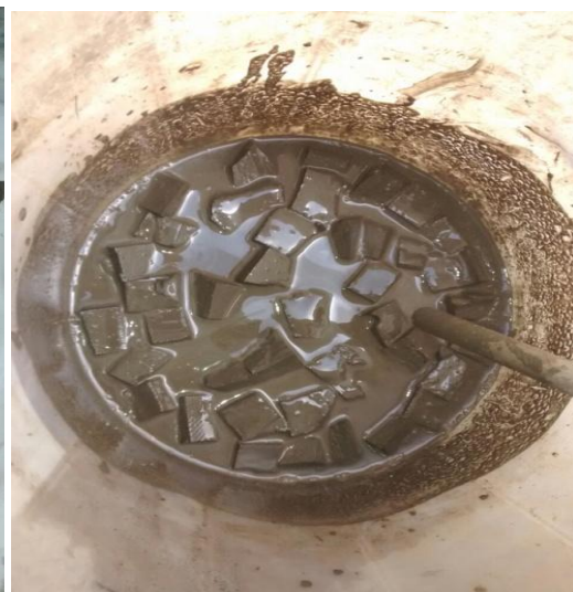
Figure 1: NaOH treated rubber. Figure 2: Cement paste treatment given to rubber.
