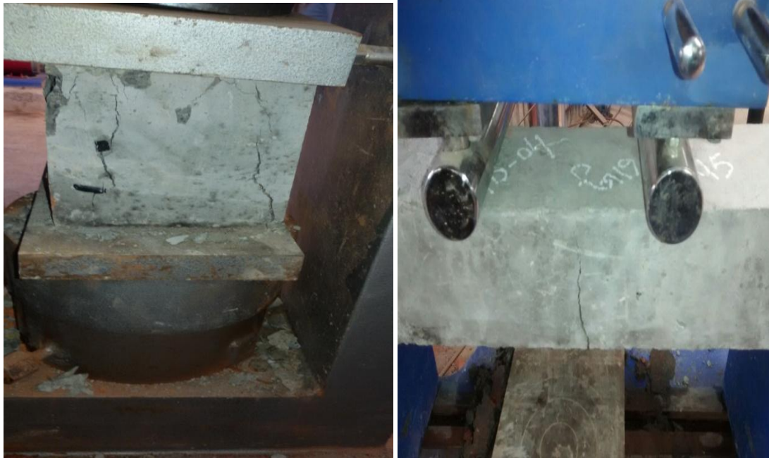
Figure 3: Compressive Strength Test on Cube Specimens Figure 4 : Flexural Strength Test
