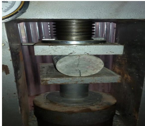
Figure 5: Split Tensile Strength Test
