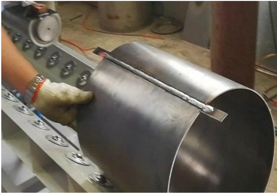
Figure 2: The custom developed boiler cylinder
