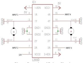
Pin configuration of Driver Circuit
