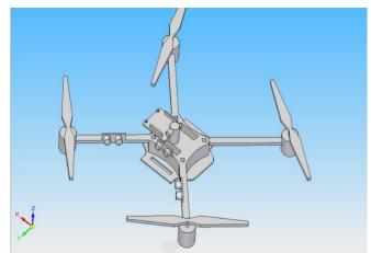
Top View of the drone and bird repeller system
