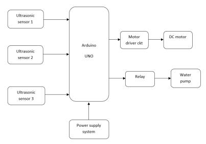
Block diagram of bird repeller system
