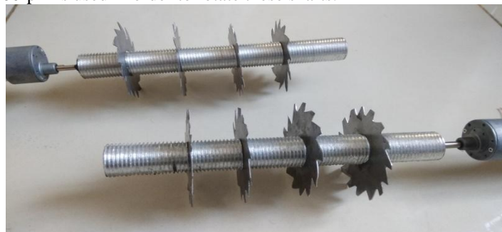
Fig 3.2: Cutting discs attached with rotating shaft
