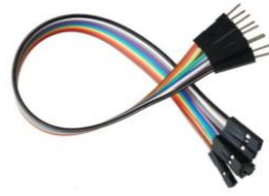
Fig-8: Jumper Wires
