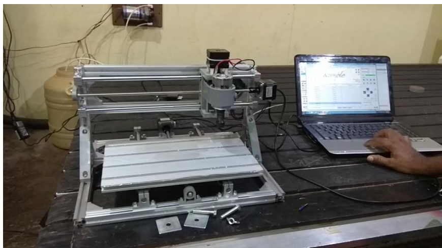
Fig 21. Working setup laptop with fabricated mini CNC route
