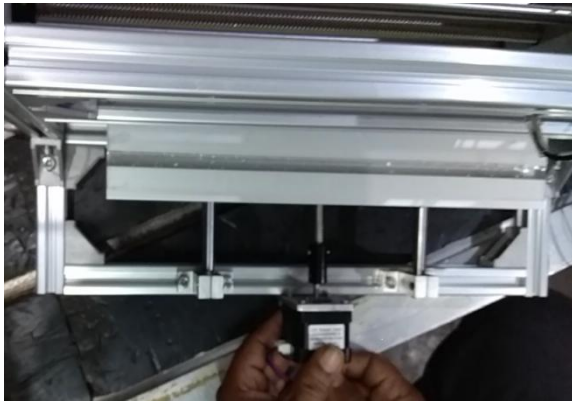
Fig 18. Stepper motor mounting on XY axis
