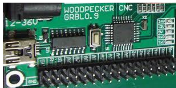
Fig 7.Arduino nano microcontroller in grbl0.9i control board
