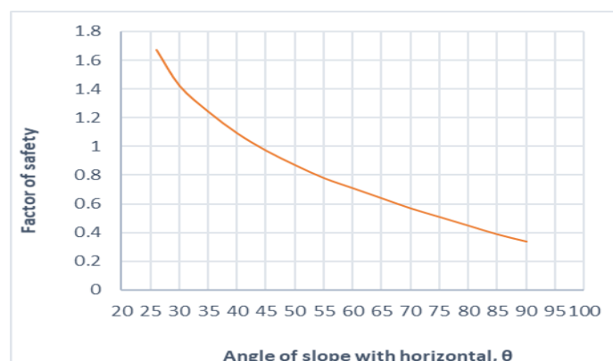
Fig. 1 Graph of FOS versus angle of slope with horizontal
