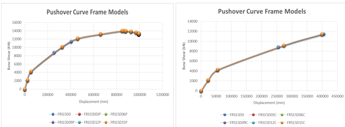
FIGURE 6 Pushover Curve of 15 Storey Frame Models
