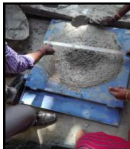
Fig2 SLUMP FLOW TEST
