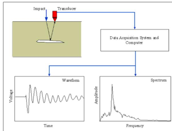
Fig. 2 schematic diagram of working of IE
