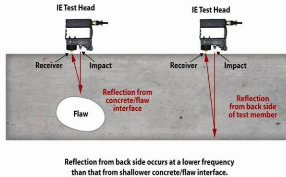
Fig. 1 shows the working of IE the stress wave reflects from the surface of flaws of the concrete
