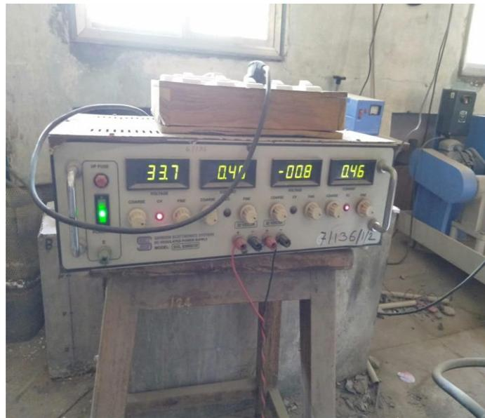
*Fig.5 Accelerated corrosion assembly*
