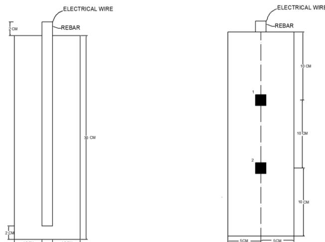
*Fig. 4 Specimen size and rebar position*
