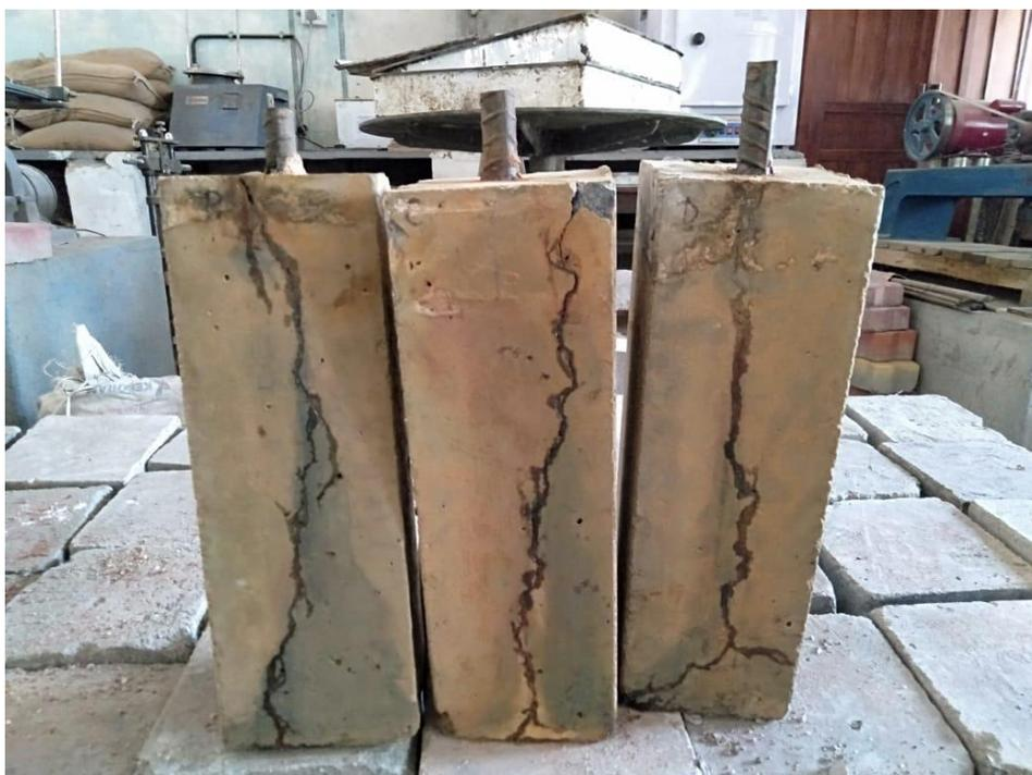
Fig 6. Cracked beam specimen
