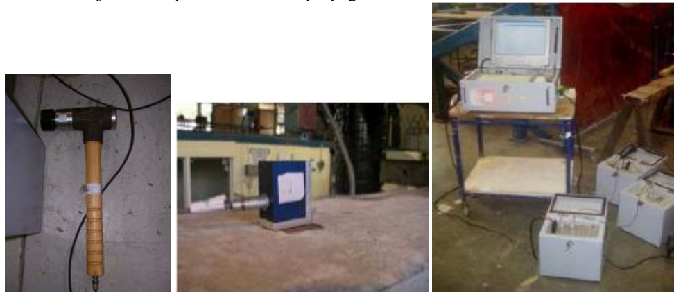
a) Impact hammers b) Accelerometer c) Unit boxes and computer
