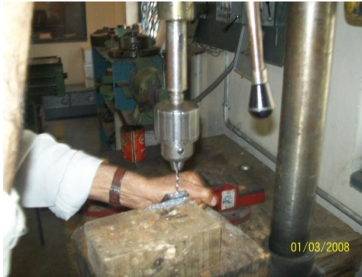
Fig.10: Holes drilled on the groove perpendicular to the cut
