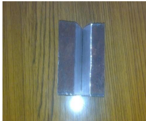
Fig.2: Single V-butt samples without holes
