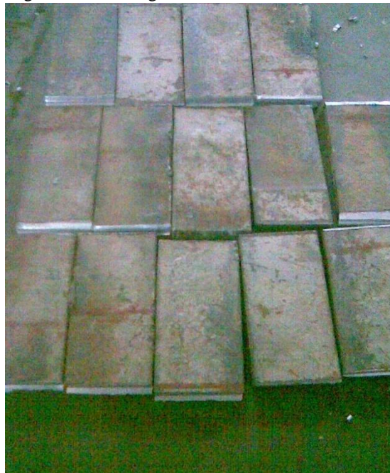
Fig. 9: Single V-grooved samples ready for welding
