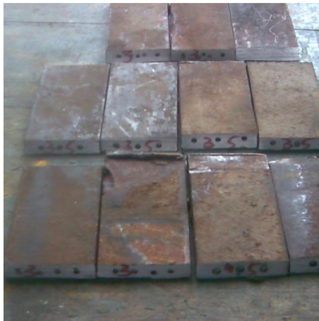
Fig.11: Single V-grooved samples with holes for welding.
