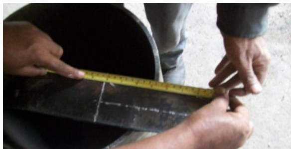
Fig. 5: Measurement and marking of the sample
