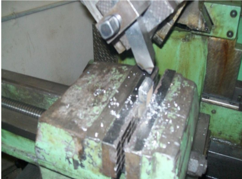
Fig. 8: Edge cutting at an angle of 30^\circ with sample surface
