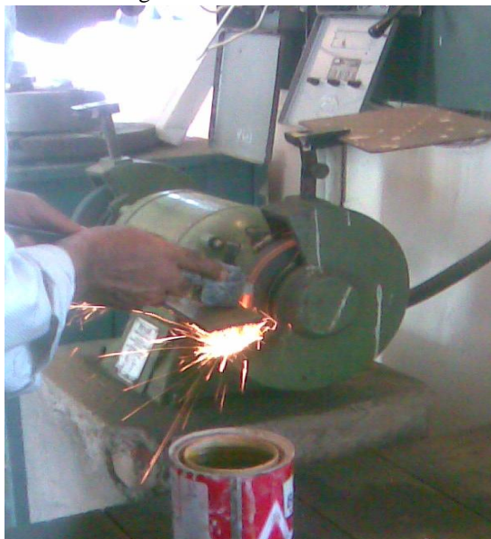
Fig.7: Grinder on sample pieces for smooth surface
