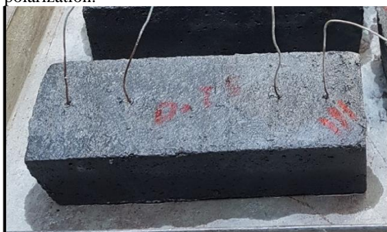
Fig. 3. Cement mortar mould with four copper wires
