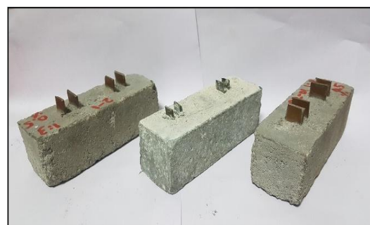
Fig. 4. Cement mortar mould with four copper plates
