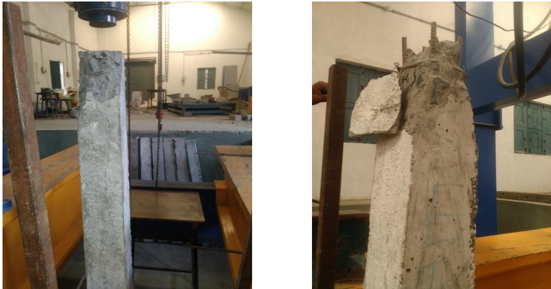
Fig. 9 Control column failure
