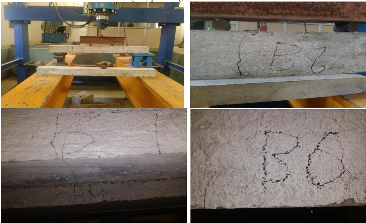
Fig. 4 Creating control damage to columns
