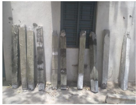
Fig. 10 Failure of wrapped columns
