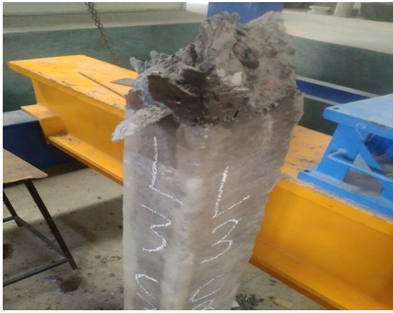
Fig. 10 Failure of wrapped columns
