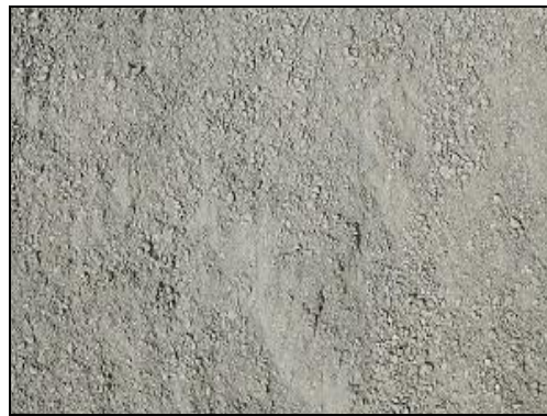
Fig. 5 Appearance of stone dust
