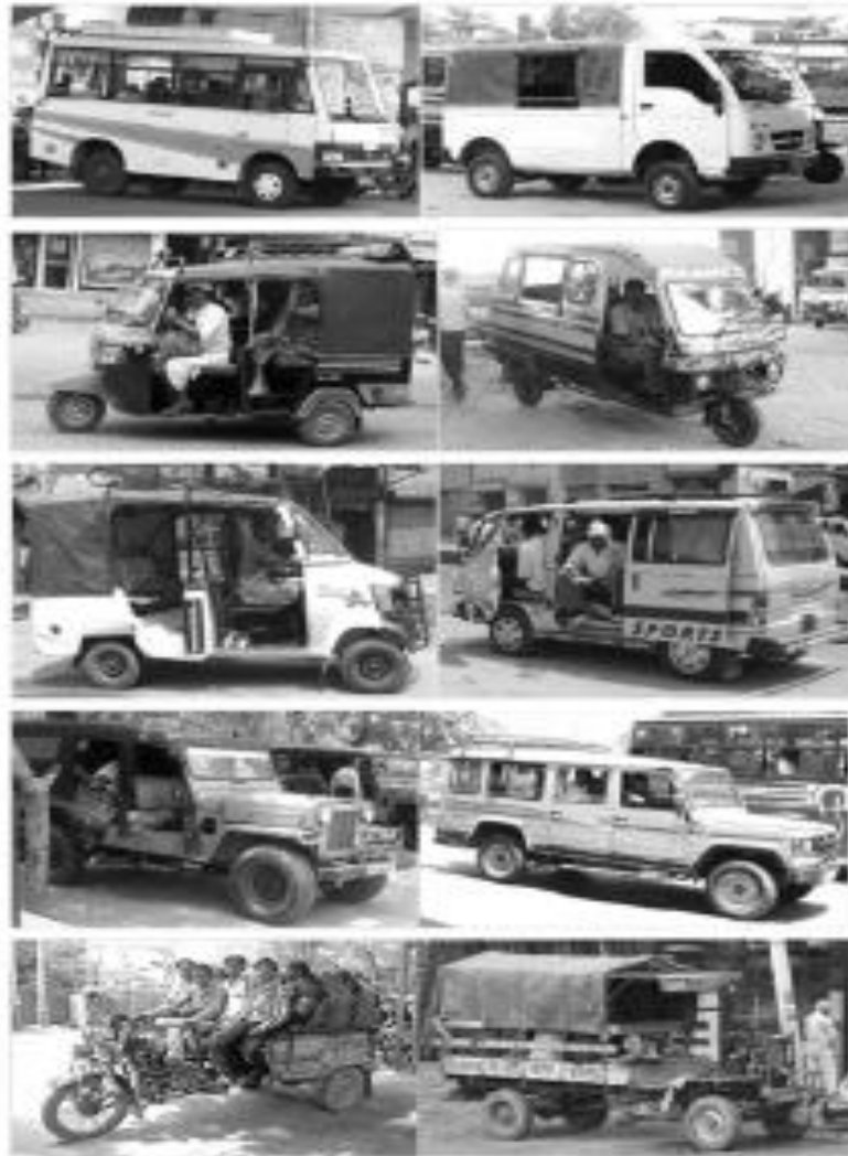
Fig. 2. Photographs of typical informal public transport modes studied in the target cities/city regions (Left to right, top to bottom: Minibus, Tata Magic, Auto-rickshaw, Vikram, Mahindra Gio, Maruti Omni, Jeep, Force Cruiser, Chakda, Kaduka). Source: M. Kumar et al.
