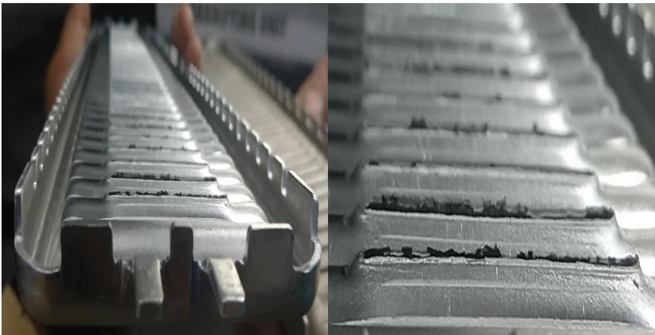
Figure 6 Heavy burrs on slots of header plate
