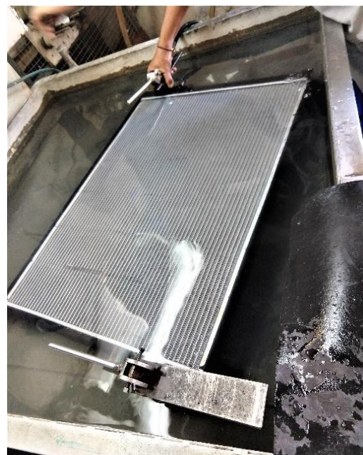
Figure 3 Wet leak test
