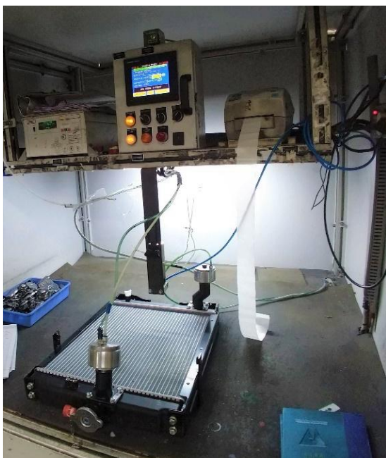
Figure 2 Dry leak test
