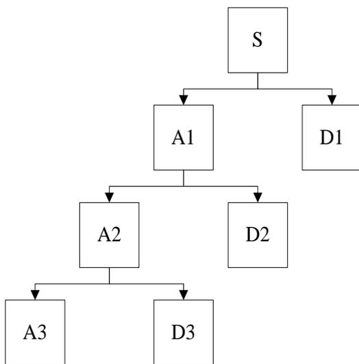
Fig 1. Wavelet decomposition tree [7]
