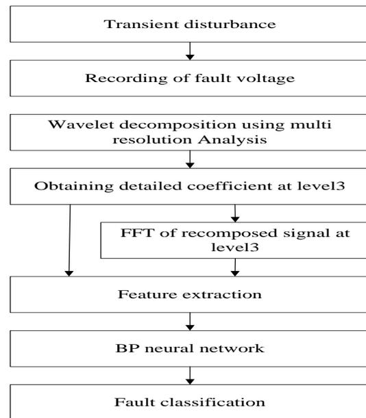
Fig 2. Procedure of Fault analysis [7]
