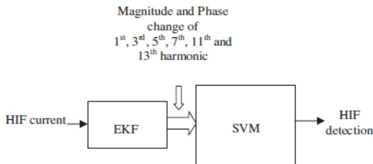
Fig 3. Proposed HIF detection scheme [16]
