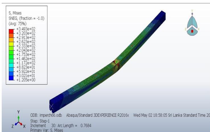
Fig.7 Von Mises Stress Contour for Ch48
