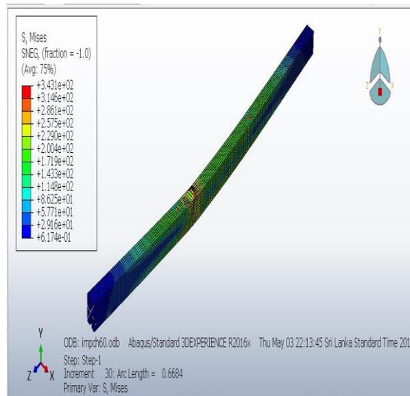
Fig.9 Von Mises Stress Contour for Ch60
