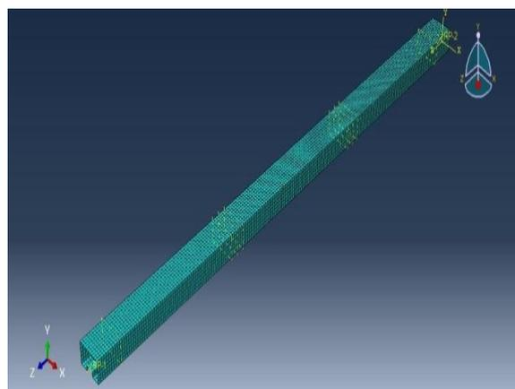
Fig.4 Meshing of Hollow Channel section
