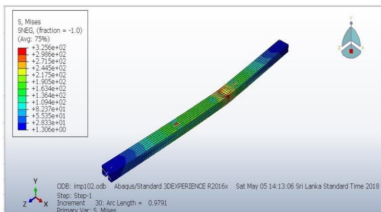
Fig.12 Von Mises Stress Contour for Ch102
