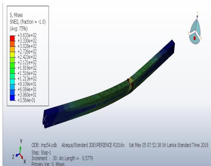
Fig.8 Von Mises Stress Contour for Ch54
