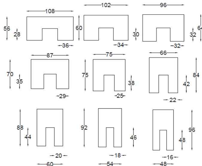
Fig.2 Geometry of the proposed Hollow Channel sections
