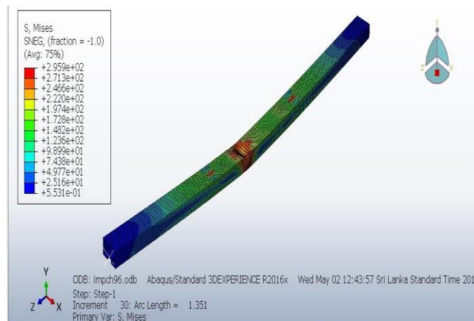
Fig.11 Von Mises Stress Contour for Ch96
