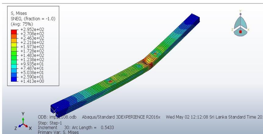
Fig.13 Von Mises Stress Contour for Ch108
