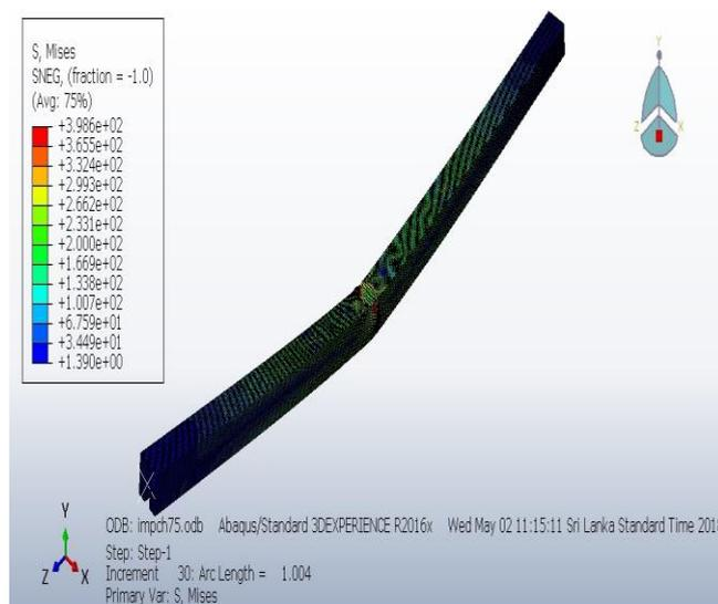
Fig.5 Von Mises Stress Contour for Ch75
