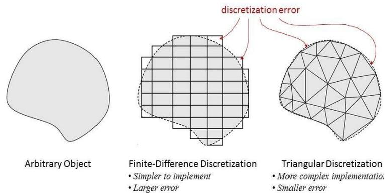
Fig.1 Finite Element Discretization
