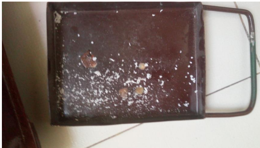
Fig. 4 Ash formed after pad burning
