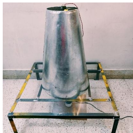
Fig 2.5: Assembled Solar Updraft Tower.
