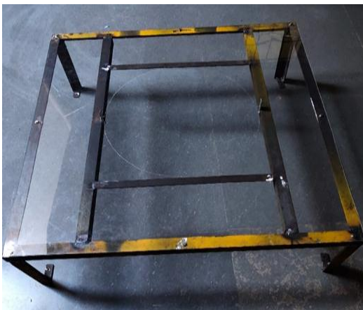
Fig 2.2: Collector Plate (Acrylic sheet) placed on a metal frame.
