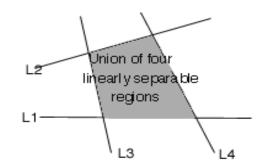
Figure .2.4 Intersection of 4 linearly separable regions forms the center region.
