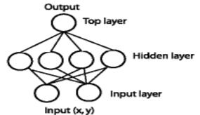
Figure 2.2. A feed-forward network with one hidden layer.
