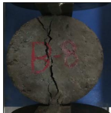
(b) Crack pattern at the final failure
