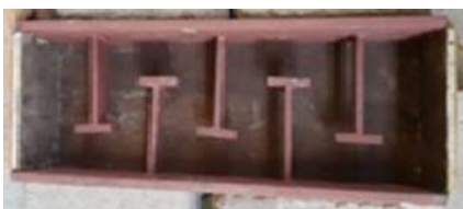
Fig.7 Mould of SCS beam with T-Connectors
