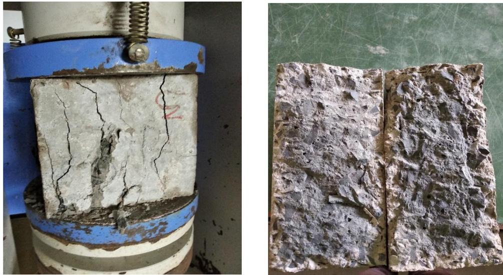
Figure 11: Failure of specimen
