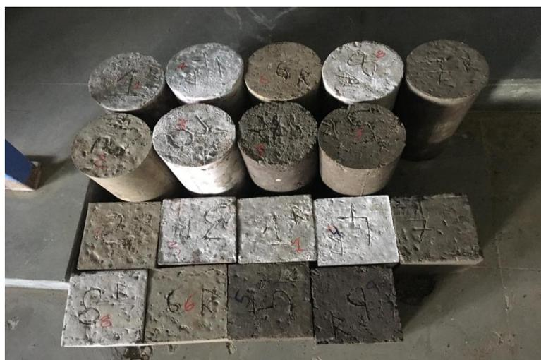
Figure 10: Curing of specimen
