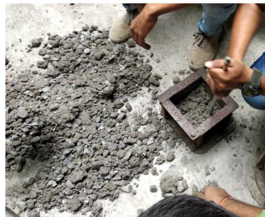
Figure 9: Placing concrete
