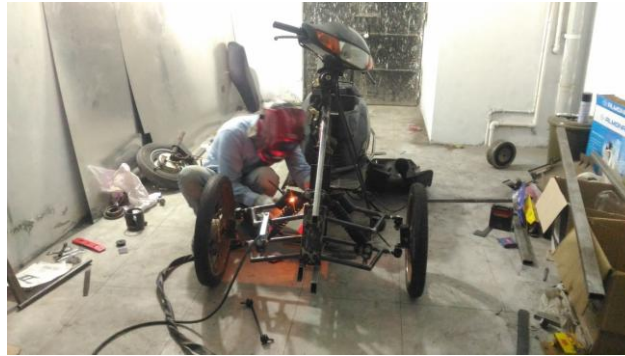
Fig. 18 Installation of tie rods, steering rod and wheels
