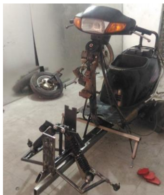
Fig. 17 Installation of control arms, suspension stand and shock absorbers on body frame
