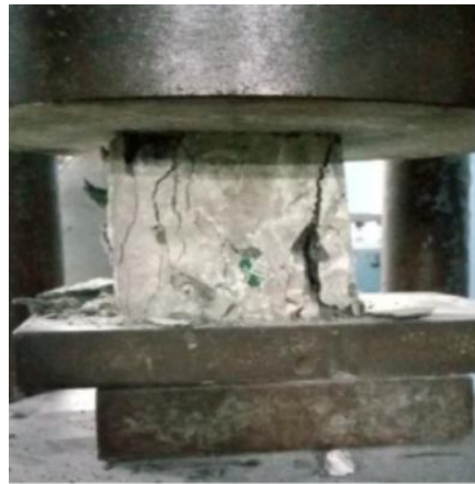
Fig .7 Testing and failure pattern of cube
