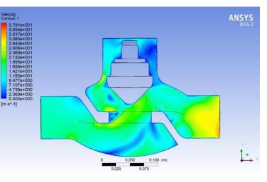
Figure 7: CFD result trial-3 velocity contour
