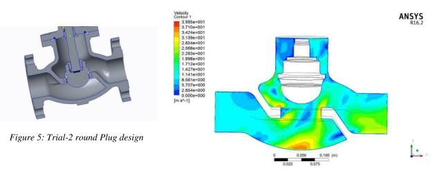
Figure 5: CFD result trial-2 velocity contour
