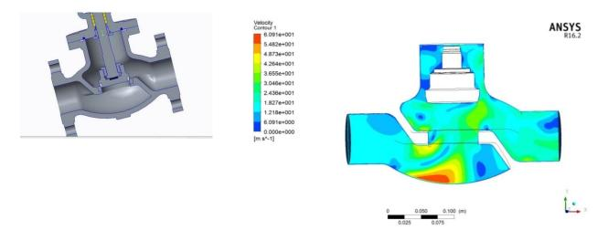
Figure 4: Trial-1 Flat Plug design
