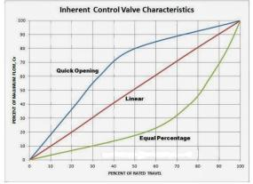
Figure 1: Flow characteristics
