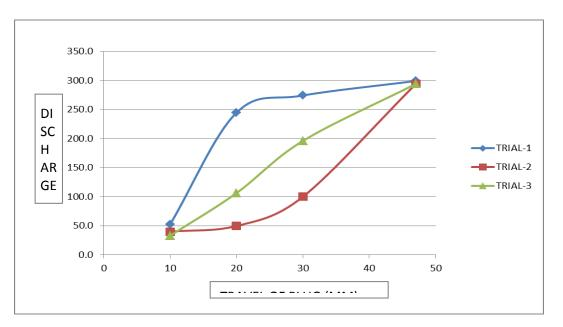
Figure 8: Discharge VS Lift Characteristic curve
