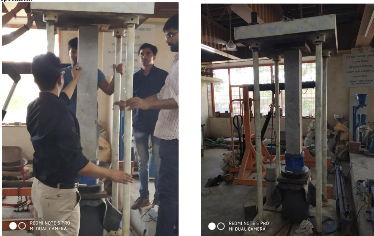
Figure 4&5 Testing Setup of Loading Frame
