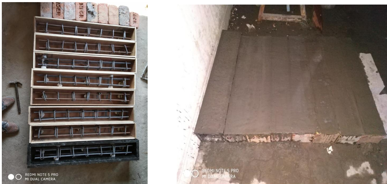
Figure 2&3 Casting of Column specimen (size 150 X 150 X 1000MM)
