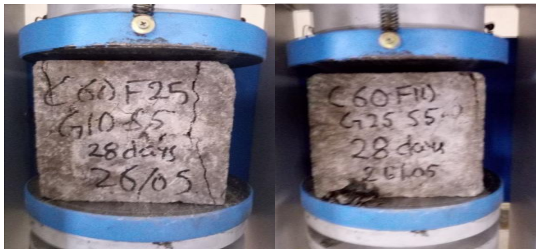
Figure 3: Failure of quaternary blended concrete with 40% replacement
