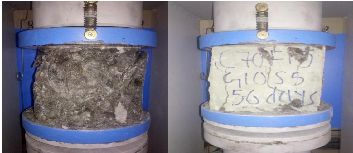
Figure 2: failure of 100% OPC concrete and quaternary blended concrete with 30% replacement
