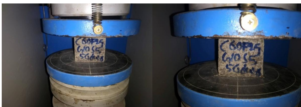
Figure 5: Compressive strength and failure of 40% replacement of cement with SCMs in quaternary mortar
