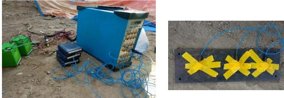
Figure 2 Instrument setup: OROS OR36 analyzer
