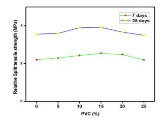
Fig. 6. Relative Split tensile strength of concrete mixtures
