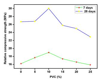
Fig. 4. Relative compressive strength of concrete mixtures
