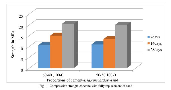
Here we take only 2 proportions of cement and slag and then sand is totally replaced by crusher dust. From this we got that by fully replacing the sand with crusher dust we cannot achieved the target strength of the cubes.
