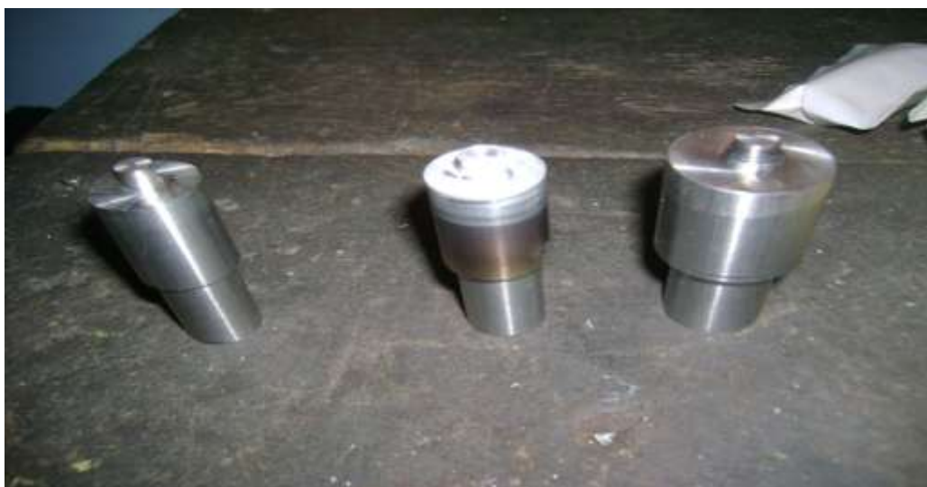
Figure 04 Tools used for friction stir welding process
