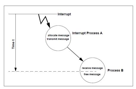
Figure 1. Real-Time System Definition [5]
