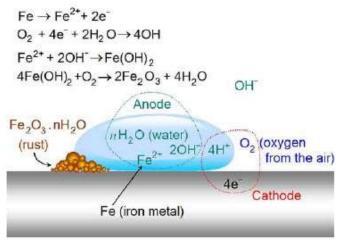
Fig.2 Corrosion process
