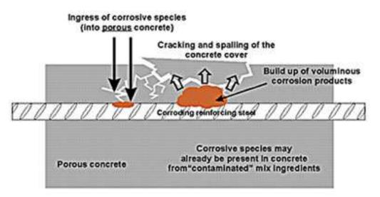
Fig 1. Corrosion of Reinforcement
