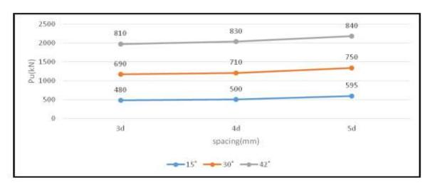
Fig. 1.-Ultimate Load Vs Spacing Between Piles for 3x3 Pile<sup>[1]</sup>
