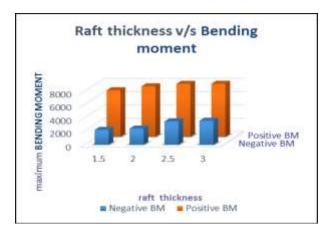
Fig.3 Raft thickness v/s bending moment<sup>[3]</sup>
