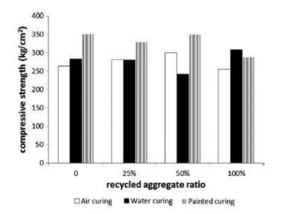
Figure 3 Compressive strength for various recycled aggregate
