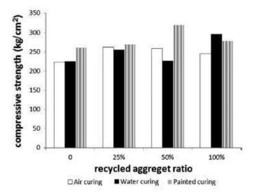
Figure 2 Compressive strength for various recycled aggregate ratio at 7 days.
