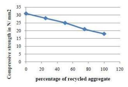
Figure 4 compressive strength of recycle aggregate at 28 days
