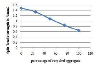
Figure 5 Tensile strength of recycle concrete aggregate at 28 days
