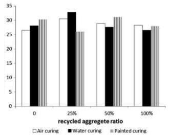
Figure 6 Tensile strength of recycle concrete aggregate at 28 days
