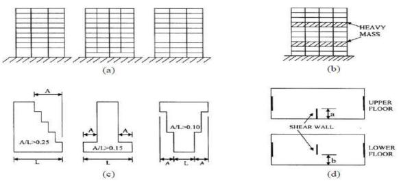
*Figure* <sup>[1]</sup>(*a*) *Stiffness/strength irregularity;*
