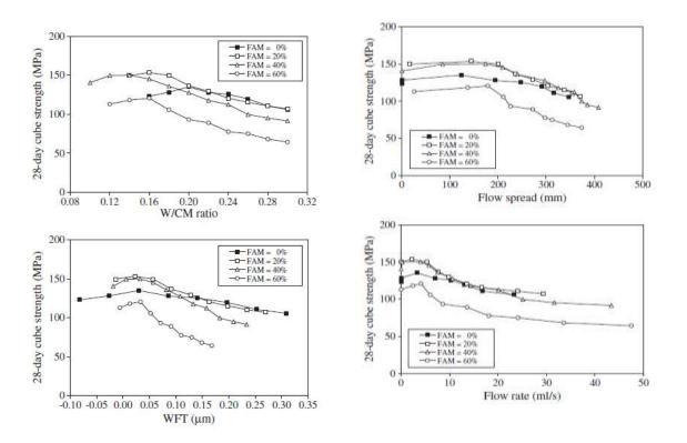
Figure 1 - cube strength versus W/CM ratio and WFT
