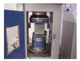
Figure 6 Compressive test
