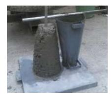
Figure 7 Workability test
