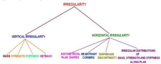
Figure 1.1 Classification of different types of structural irregularities (https://image.slidesharecdn.com/organizationalstructure)
