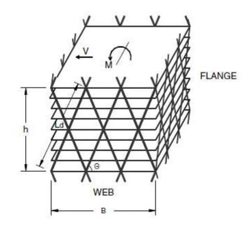
**Figure 2 Typical Diagrid Module**
