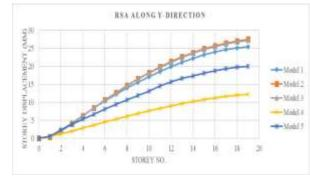
Figure 6 Response Spectrum Analysis of storey displacement in Y-direction
